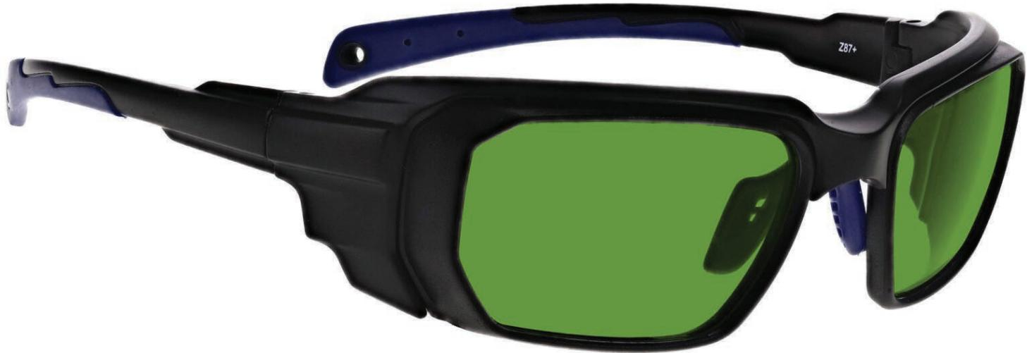
The D1500 laser safety glasses have a polycarbonate green lens filter that provides laser protection. These laser glasses have visible light transmission of 16%. In addition, the D1500 laser safety glasses have ANSI Z87.1 and ANSI Z136.1 safety standards. These laser safety glasses 16001 is a durable and lightweight wrap around frame. Made of high-quality plastic, the 16001 laser safety glasses feature adjustable nosepads. These Phillips Safety laser safety glasses are available in black/blue.
